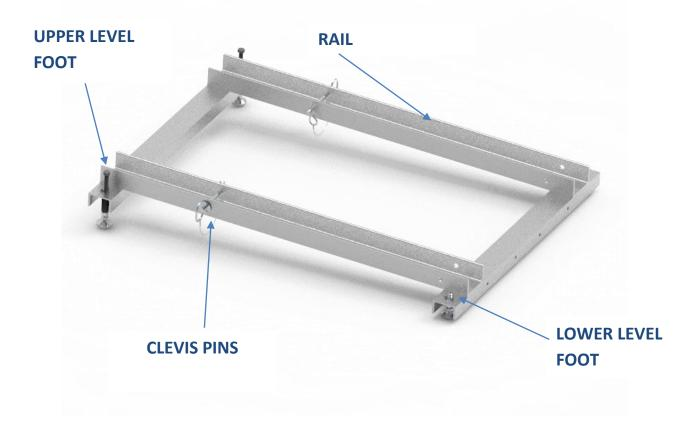
The Single Rail Assembly is intended to be operated as a base to adjust the operating angle of one TR-2 Trimmer. The Primary Rails are intended to hold the wheels of one trimmers. The Clevis pins ensure the unit does not roll off of the Rail Assembly. The Upper Feet allow the operator to adjust the angle of operation of the trimmers.
